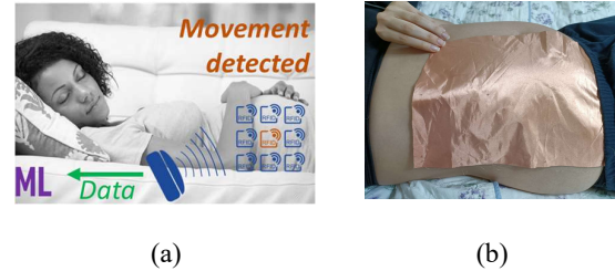
Figure 1. (a) Concept of the RFID system for monitoring fetal movements. (b) A woman in the 24 th week of pregnancy wearing the ground plane of the grid.
