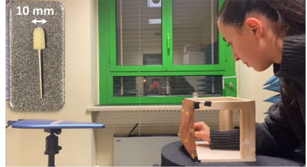
Figure 4. Picture of the grid interrogation while one tag was displaced to reproduce a kick of a 20-week-old fetus. In the inset: the cylindrical probe which reproduces the fetal foot.
