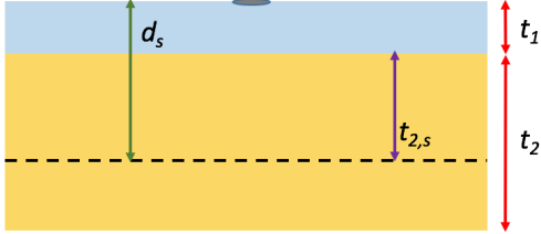
Figure 4. Diagram of the heterogeneous sample, composed of Material 1 (top, blue) and Material 2 (bottom, yellow). The probe position is indicated by the grey oval. The sensing depth, d_s , and thicknesses of Material 1 ( t_1 ) and Material 2 ( t_2 ) are indicated. Also shown is t_{2,s} , the thickness of Material 2 that is within the sensing depth.
