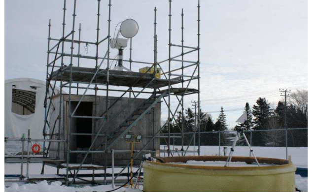
Figure 2. Normalized radar cross section (NRCS) measurements of the circular oil-in-sea ice tank through a C-band scatterometer. A trihedral calibration is performed in this scene.
