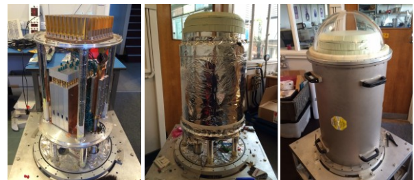
Figure 9. PHAROS cryostat (a) no heat shield and IR filter, (b) with heat shield and IR filter, (c) fully assembly with Plexiglas and outer shield.
