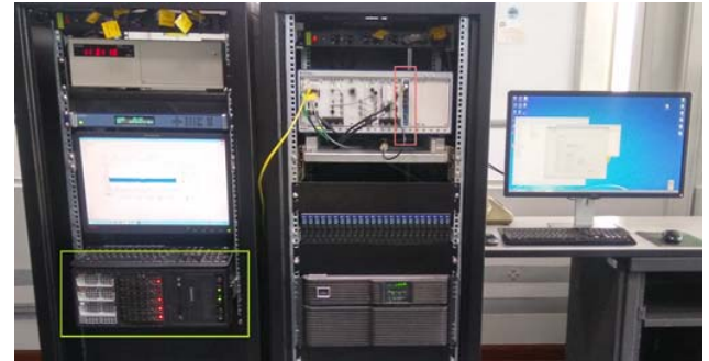
Figure 3. Control room at the Institute for Radio Astronomy. The FlexRIO receiver module indicated by the red rectangle is directly connected to the FPGA module, which cannot be observed because it is installed inside the PXIe chassis. The NIXSYS server (64 cores, 64 GB of RAM) is indicated in green.
