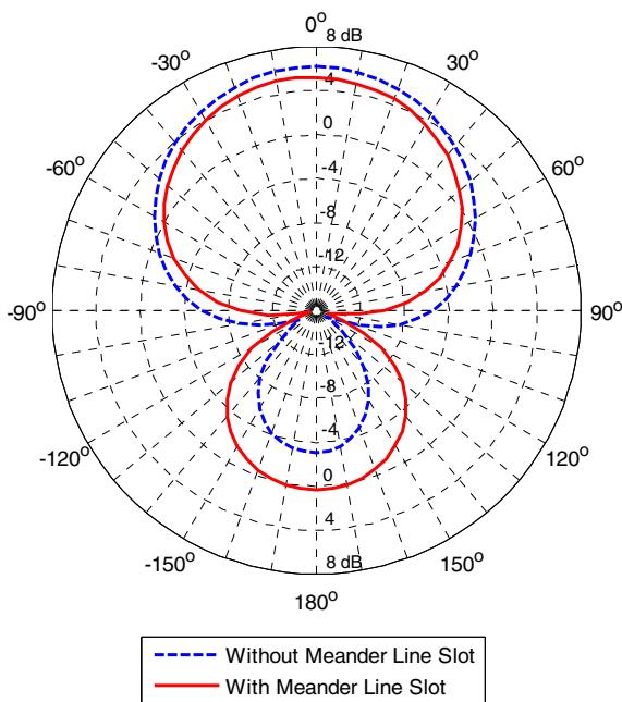
**Figure 3.** Comparison of Radiation Pattern
