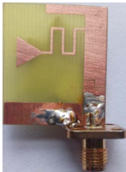
Figure 8. Fabricated prototype of the intended tri-band MTM antenna.
