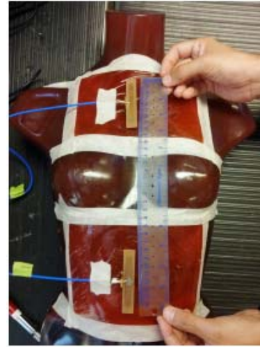
Figure 4. Placement of antennas over the phantom for Case-II.
