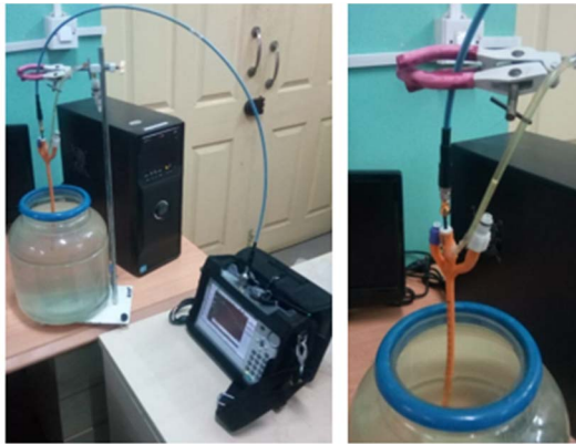
Figure 5. Experimental setup showing the applicator supported with clamps inserted inside water bath with connecting cables to vector network analyzer.
