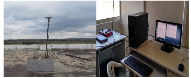
Figure 1. Septentrio PolaRxs-Pro GNSS receiver and antenna setup at GCET, Hyderabad
