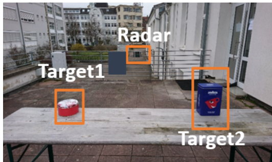
Figure 5. Experiment setup to measure effects of adverse weather conditions. Two targets are mounted in front the radar that is mounted in a box with additional sensors such as a camera. The radar radome was exposed to different water applications representing drizzle or splash water.
