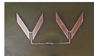
Figure 2. Fabricated two element array comprising of two V-shaped patch elements
