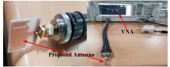
Fig .4. Antenna under test using VNA
