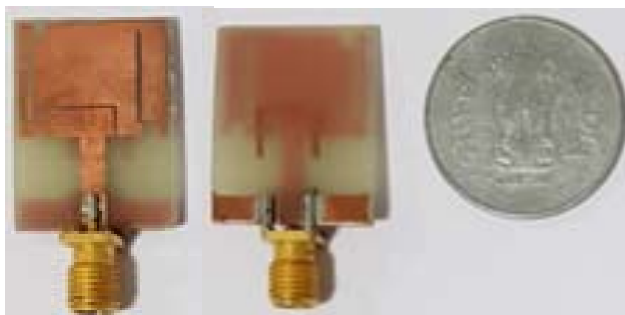
Fig .3. The fabrication prototype of proposed antenna top and bottom view.
