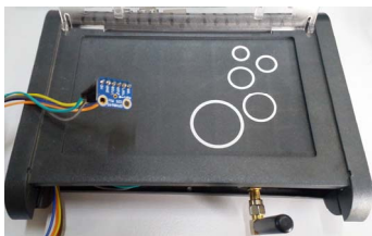
Figure 1. Device with microphone developed for voice messaging
