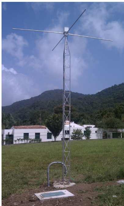
Figure 2. An antenna and tower similar to those to be used for the Aguadilla Radio Array. The dipole elements are 1.8 meters from end to end. The small box above the antenna contains the preamplifier.
