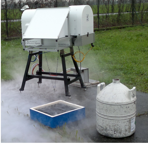
Figure 1. The radiometer installed at the experimental station of Spino d'Adda, during cold load calibration.
