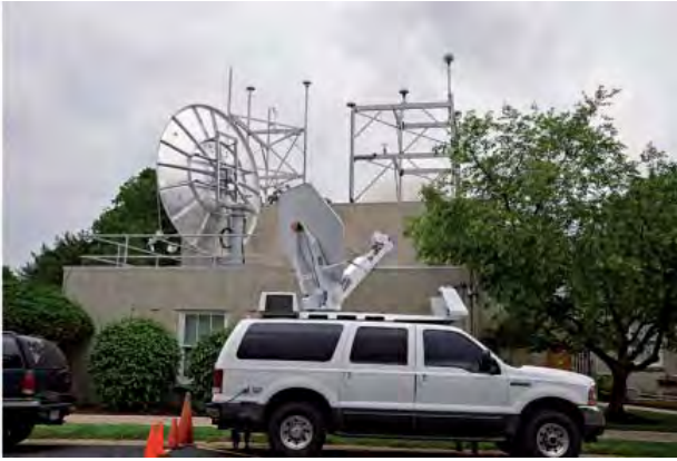
Figure 13. A portable two-way satellite time and frequency transfer (TWSTT) station, which is driven to remote sites for the purpose of calibration. The raised antenna ensemble on the taller roof is designed to minimize multipath. The large dish on the roof is capable of providing digital uplink information for GNSS systems, or conducting high-SNR two-way satellite time and frequency transfer observations.
