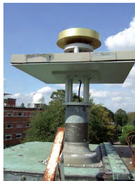
Figure 8. A GNSS antenna at the Royal Observatory of Belgium, designed with an underneath RF absorber to prevent near-field multipath.
