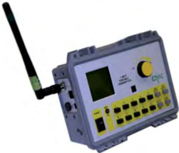
Figure 1. A typical transmitter used to generate the CW signal.
