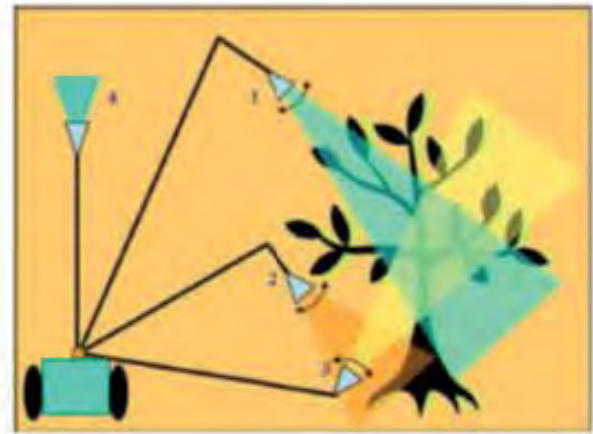
Figure 12. A schematic drawing of the microwave measurements of [70]: (1) downward (soil + trees), (2) downward under crown (soil), (3) upward (trees), (4) sky [65].
