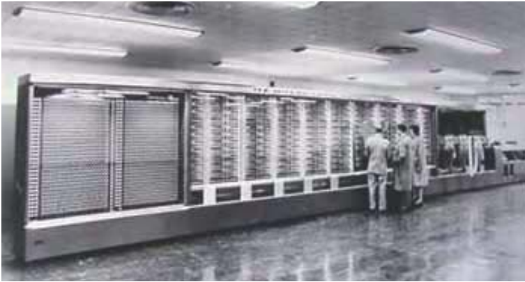
Figure 1a. The ASCC was a massive (51 ft × 8 ft) electromechanical calculator developed by Howard Aiken (Professor of Applied Mathematics at Harvard), his staff, and IBM engineers between the years 1939-1944. The Mark I was capable of addition, subtraction, multiplication, division, computing transcendental functions, and storing results for later computations via a set of 24 electromechanical storage wheels. The ASCC processed information sequentially as opposed to the parallel approach commonly used in that time period, a trend that continued for future generations of computers (photo taken from the “IEEE Global History Network” Web page).
