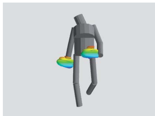
Figure 4. Two views of the cylindrical body model with the perturbed antenna.
