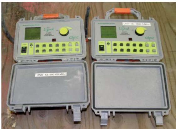
Figure 4c. A typical transmitter for the higher frequency band.
