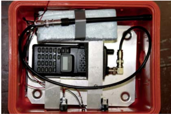
Figure 4a. A close up of a typical transmitter for the lower frequency band.
