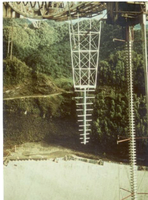
Figure 2. The log-periodic VHF feed antenna (45 MHz to 55 MHz).
