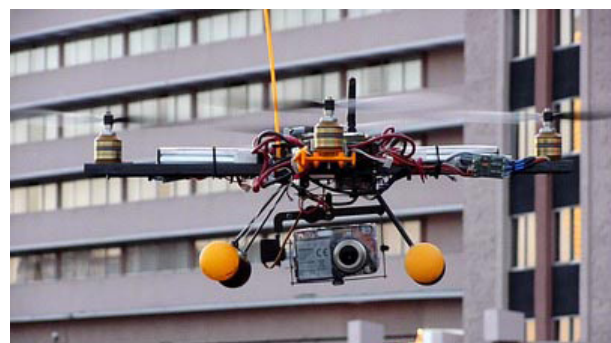
Figure 10c. The Faucon Noir UAS in flight, equipped with one of its mapping payloads.
