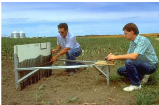
Figure 2c. An example of manual mapping methods: Measuring the linear profile of the ground height with a contact profilometer (source: weru.ksu.edu).
