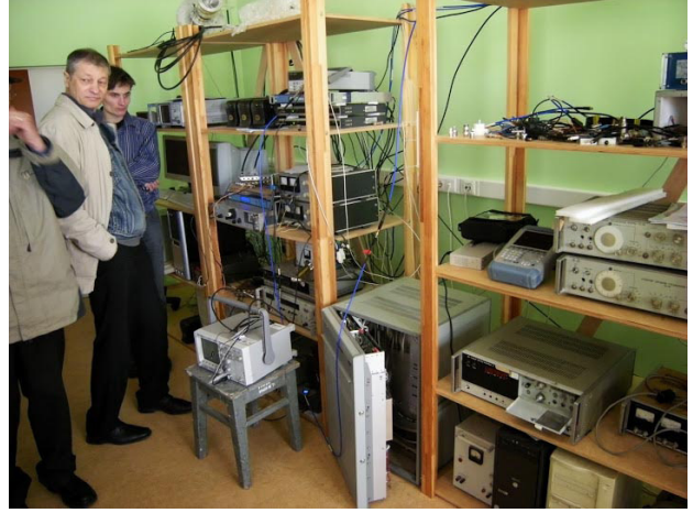
Figure 5. This shows parts of the new receiver system. The timing and frequency control are provided by a hydrogen maser (center) (photo: Joakim Johansson).
