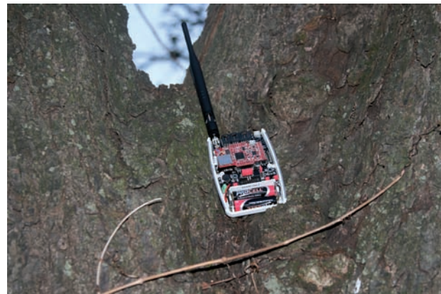
Figure 5. An example of an autonomous wireless sensor node placed on a tree (open to show the interior) (photo: M. Zennaro)
