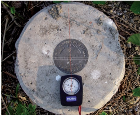
Figure 7. Geographic compared to magnetic north at El Baúl.
