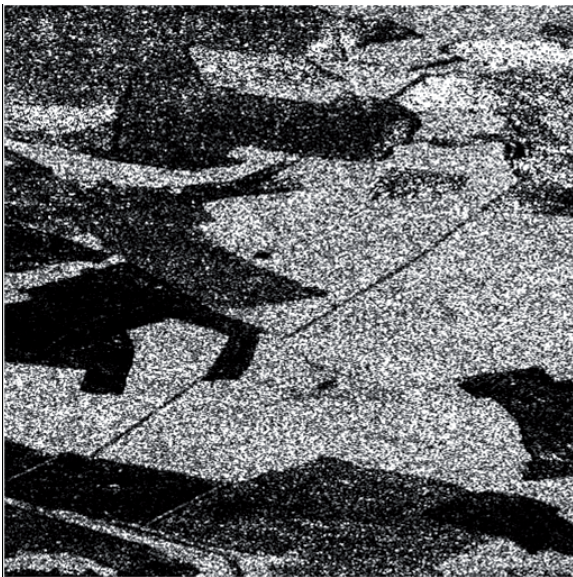
Figure 4. The SPAN image of the PolSAR data acquired by the SIR-C/X SAR system.
