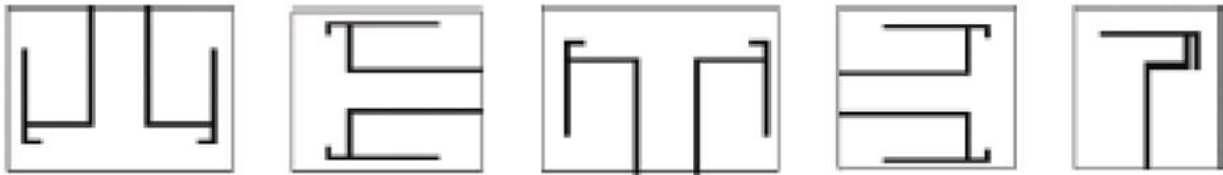
Figure 12. The orientation of the printed IFA on the body for a front view of the body: the four antennas on the left are the receiving diversity antennas, and the antenna on the right is the transmitting antenna on the belt, with \hat{a} = -\hat{y} for the belt-chest, belt-head, and belt-back channels, \hat{a} = -\hat{z} for the belt-wrist channel, and \hat{a} = \hat{y} for the belt-ankle channel.
