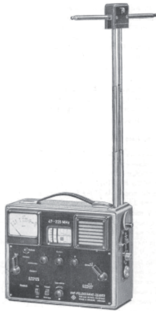
Figure 1. A photograph of the Rohde and Schwartz VHF field-strength indicator.
