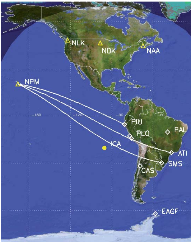
Figure 1. SAVNET stations (diamonds) and some of the transmitters used in our studies (triangles), along with some VLF propagation paths.
