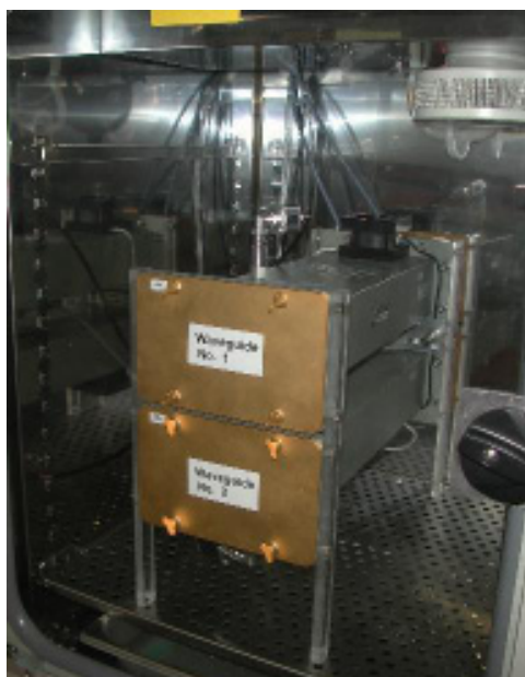
Figure 6. Rectangular waveguides shortened at one end, operating at typical frequencies of mobile communication standards [27].
