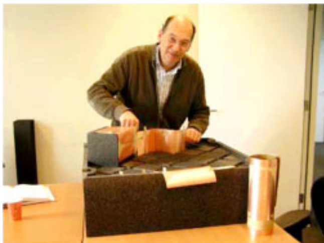
Figure 7b. An assembly of experimental printed versions of the Vivaldi elements.
