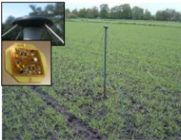
Figure 6a. An example of sparse aperture array technology from the LOFAR telescope (ASTRON): A polarization pair of “droopy dipoles” that operate from 30–80 MHz. The inset shows the low-noise amplifier hub.
