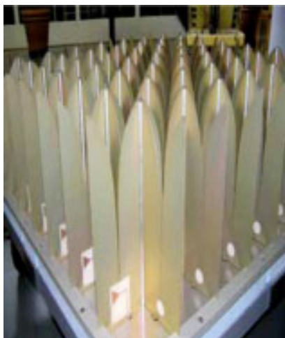
Figure 7a. Prototype dense aperture array elements for the EMBRACE demonstrator (section 8). The elements are Vivaldi end-fire types.
