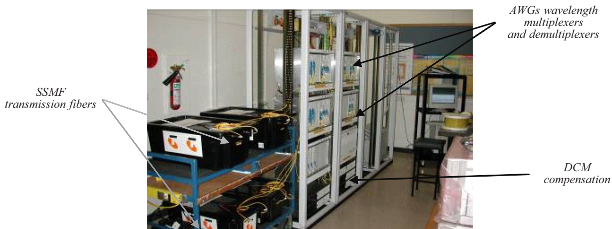
Figure 1b. Monash University Siemens TranXpress Wavelength Transport System, bidirectional 8 \times 2 \times 10 Gb/s, transmission distance 8 \times 100 km dispersion-managed (SSMF + DCMs) optically lumped amplified spans.
