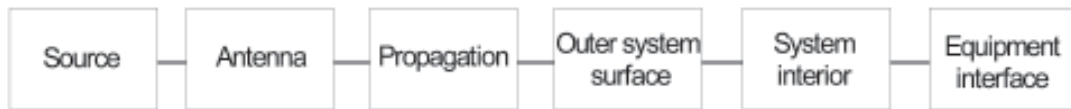
Figure 2. The factorization of the transfer function from an HPEM source to a system.
