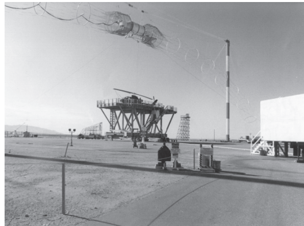
Figure 5. ATHAMAS-I: The ATHAMAS I simulator was commonly called the horizontally polarized dipole or HPD. Two 4 MV Marx generators supplied the pulsed power for this simulator.
