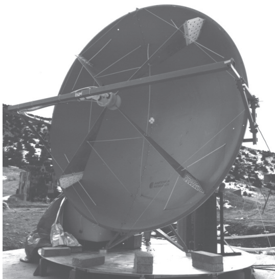
Figure 12. The IRA: The 4 m impulse-radiating antenna (IRA), built in 1994, opened up a new era in ultra-wideband, short-pulse technology.
