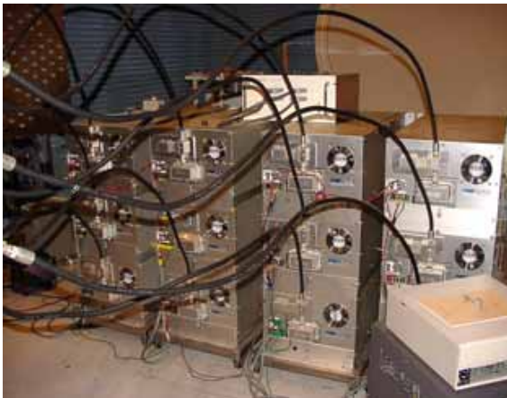
Fig.2.3.11 Phased Array with 12 Phase Controlled Magnetrons at 2.45 GHz © RISH, Kyoto University
