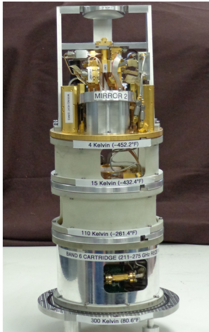
Figure 2: Picture of an NRAO-UVA Band6 ALMA receiver
