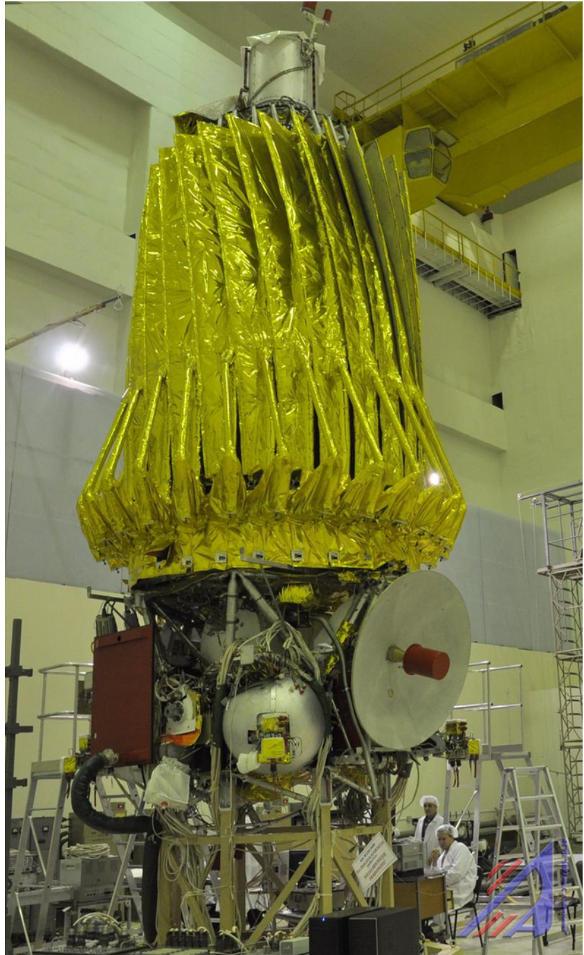
Folded Spektr-R Space Radio Telescope in the assembly complex of Lavochkin Association. Copyright: Lavochkin.
