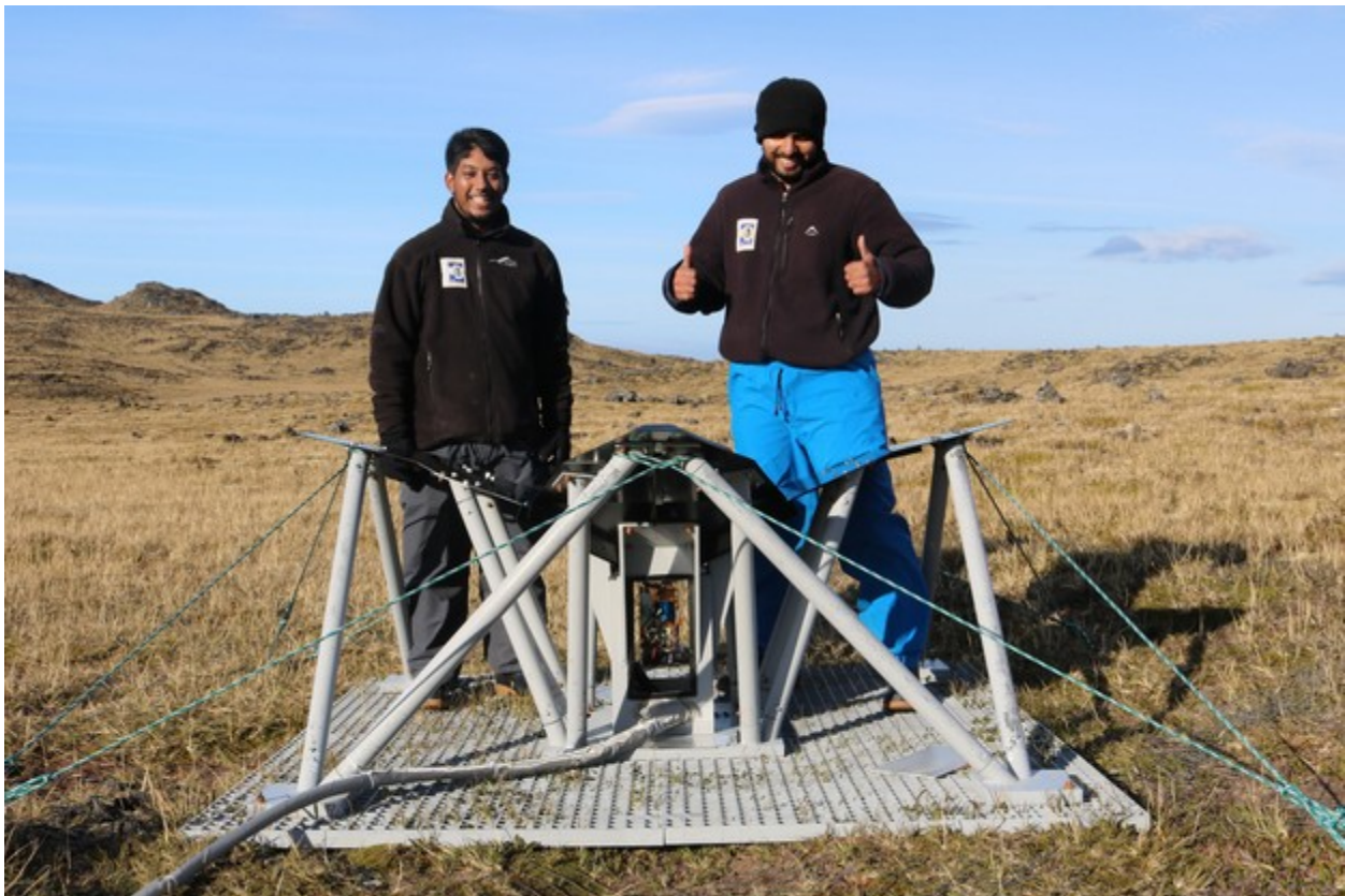
Figure 1: The PRIZM 100 MHz antenna with visible front-end electronics, newly rebuilt and installed by MSc student Nivek Ghazi (left) and PhD student Liju Philip (right).
