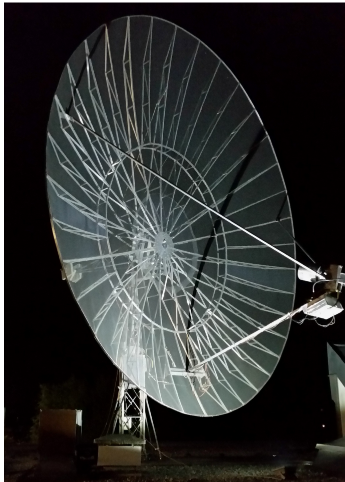
7,3m offset dish, used for receiving pulsars on 420MHz and 1292MHz
