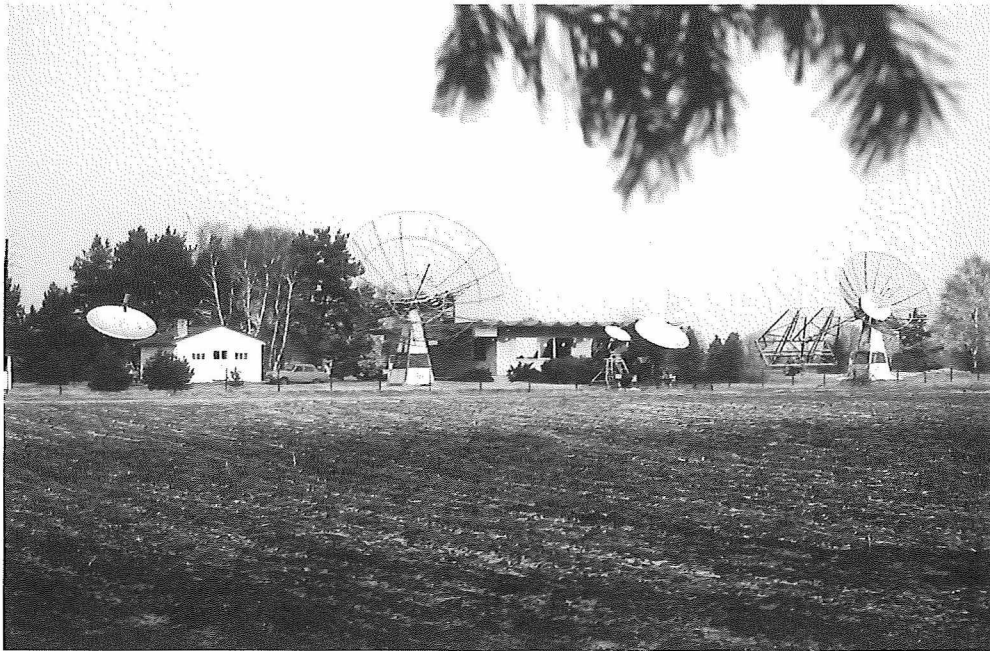
Fig. 1. View of the antenna site at the Observatory of Solar Radioastronomy in Tlemsdorf. The radio spectrograph uses three of the parabolic mirrors (10.5 m, 7.5 m, and 4 m diameter) with crossed logarithmic-periodic feeds. Observations between 40 and 100 MHz are recorded by the double-structured, logarithmic-periodic Yagi aerial in the background right of the main building. (photo: R. Engler, public relations).
