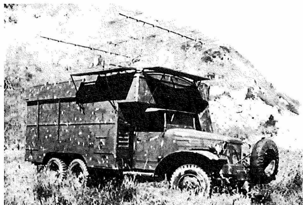
Fig. 6. LRAW radar truck with Yagis erected.
