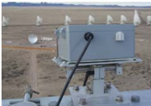
Figure 20c. A radio holography setup for the ALMA prototype antennas at the VLA site in New Mexico: the transmitter on a 50 m high tower pointed at the reflector. The VLA antennas are in the background.
