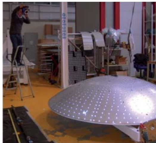
Figure 13b. The measurement setup for potogrammetry on the Large Millimeter Telescope subreflector. The camera (upper left) was moved to measure several hundred positions in three dimensions. Calibration bars are visible in the lower-left corner.
