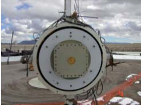
Figure 20a. A radio holography setup for the ALMA prototype antennas at the VLA site in New Mexico: the receiver feed in the prime focus box with the feed illuminating the reflector. Note the absorbent material around the feed to suppress multipath radiation.
