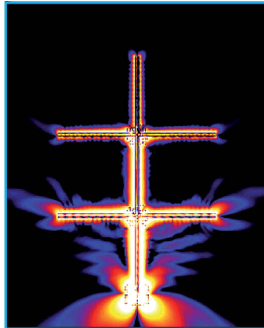
Figure 10. The power-density (dBW/sm) distribution for nano-link System 3. The color values are the same as those in Figure 6.
