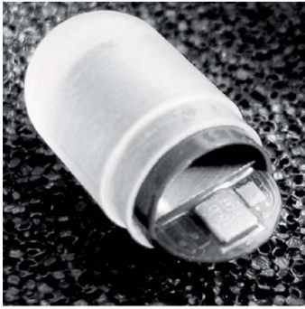
Figure 1a. The manufactured prototype of a conformal microstrip antenna by Mahe et al. [63] (©2012 Yann Mahe et al.).
