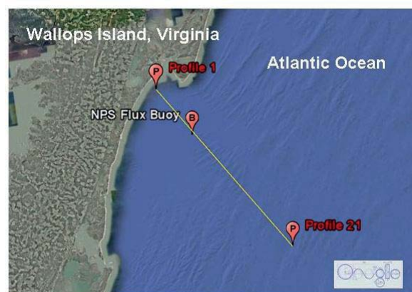
Figure 9. The propagation measurement bearing off Wallops Island, Virginia, USA, between 1512 UTC and 1605 UTC on April 28, 2000. The NPS flux meteorological buoy was located along the bearing approximately 13 km offshore.
