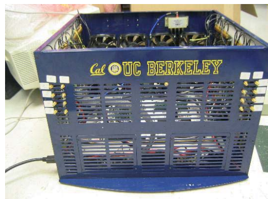
Figure 4. The IBOB/BEE2 correlator “basket” used in the eight-element Green Bank array at Galford Meadow.
