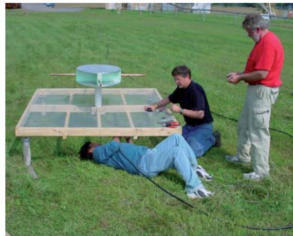
Figure 3. The antenna used in the original EoR Green Bank array. N. Biswas is shown working underneath the antenna, connecting the 50 ohm Heliax cable and power to the balun, with the author (keeling) providing instructions. Dan Boyd (standing) was preparing fasteners.
