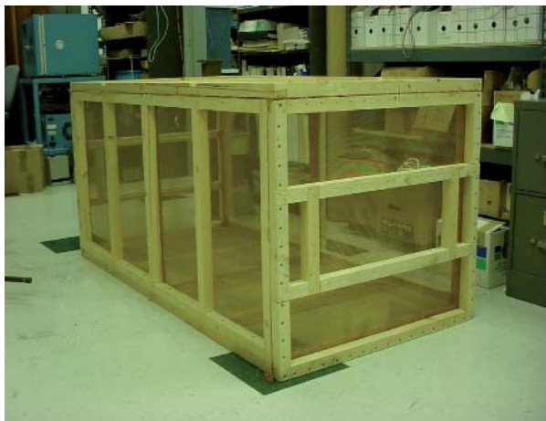
Figure 5. The EMC enclosure used to house the digital correlator. Some RF absorbing material was also required inside the enclosure, but is not shown.
