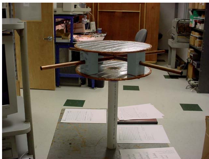
Figure 1. The original sleeved dipole prototype, used to evaluate its electromagnetic properties.
