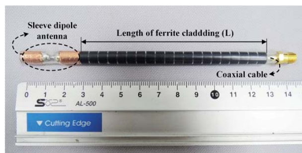
Figure 5. A photograph of the sleeve-dipole antenna fed by a coaxial cable on which the total length ( L ) of ferrite cores was clad.
