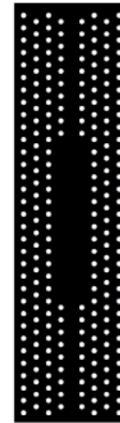
Figure 1b. The geometry of the photonic crystal considered in SOLBOX-07: A modified version that is obtained by removing further holes to form a hole-free cavity.
