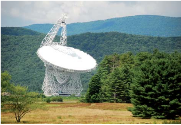
Figure 8. The Robert C. Byrd Green Bank Radio Telescope is the world's largest fully steerable radio telescope, with an aperture diameter of 300 feet (92 m). It is located at the National Radio Astronomy Observatory (NRAO), Green Bank, West Virginia, USA. The antenna beamwidth at 70 cm is 33 arc-minutes, and 5 arc-minutes at 13 cm. For comparison, the moon's angular diameter is 30 arc-minutes to 33 arc-minutes.
