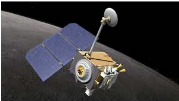
Figure 12. The Lunar Reconnaissance Orbiter (LRO), a NASA robotic spacecraft, was launched in June 2009. It is currently orbiting the moon in an elliptical 30 km by 160 km (19 miles by 100 miles) polar orbit. LRO's Miniature Radio Frequency (Mini-RF) radar instrument demonstrated new lightweight synthetic-aperture radar techniques at the moon. Although the Mini-RF transmitter failed in January 2011, it was possible to conduct bistatic lunar radar observations using the Mini-RF receiver for observing lunar radar echoes from the Arecibo transmissions.
