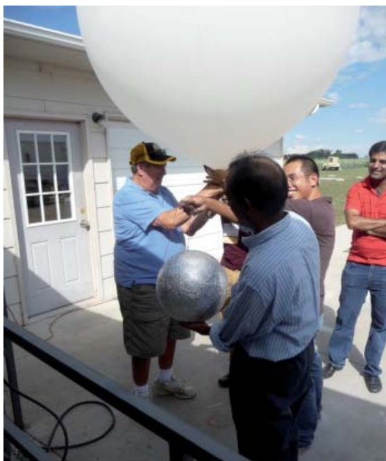
Figure 25. The preparation of a free-flying sphere for a calibration experiment at the CSU CHILL facility at the AMS Radar Calibration Laboratory in 2013.
