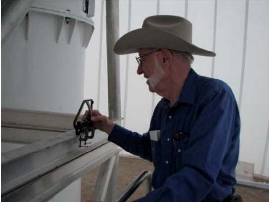
Figure 3. A gunner's-quadrant measurement on a flat surface being made by one of the authors (PLS) at the CSU-CHILL radar facility.
