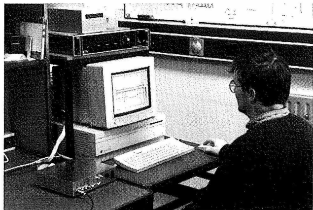
Fig 2. DSP system shown here to the left of an Apple Macintosh IIx running the application GRAFT (detailed in the following article)
