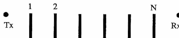
Fig 3. The N knife edges attenuate the field by a factor of 1/(N+1) .
